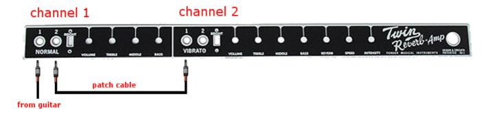
Simply plug in your guitar into the first input jack of channel 1. Run a short shielded patch cable from the second input jack of channel 1 to the first input jack of channel two and you re done !
