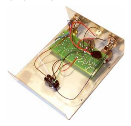
It 's easy to see if your model is true-bypass or not: if your switch has six lugs (DPDT) you have one of the older boxes and it is not true-bypass or maybe modded to true-bypass without LED indication! If your switch has 9 lugs (3PDT), congratulations - it is a newer model and factory equipped with true-bypass.
