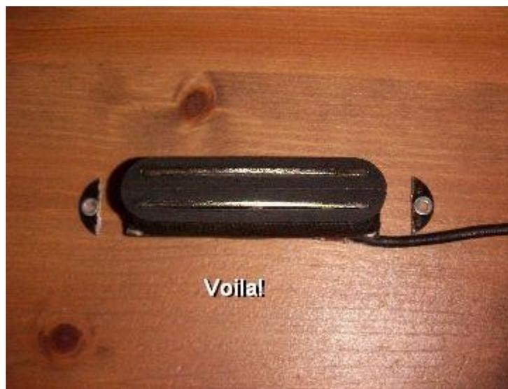
The next step is to grind the edges of the pickup (carefully!)
