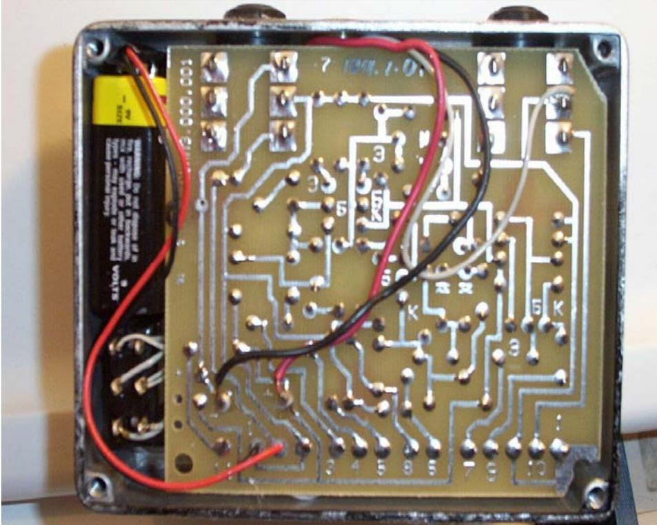
But now let's go and make the thing true bypass. The first way described here is a good way if you don't want to change the factory installed DPDT switch (6 lugs) for a 3PDT switch (9 lugs). You can also make the thing true bypass but without LED indication ! It's very simple, just follow this schematic and you're done:
