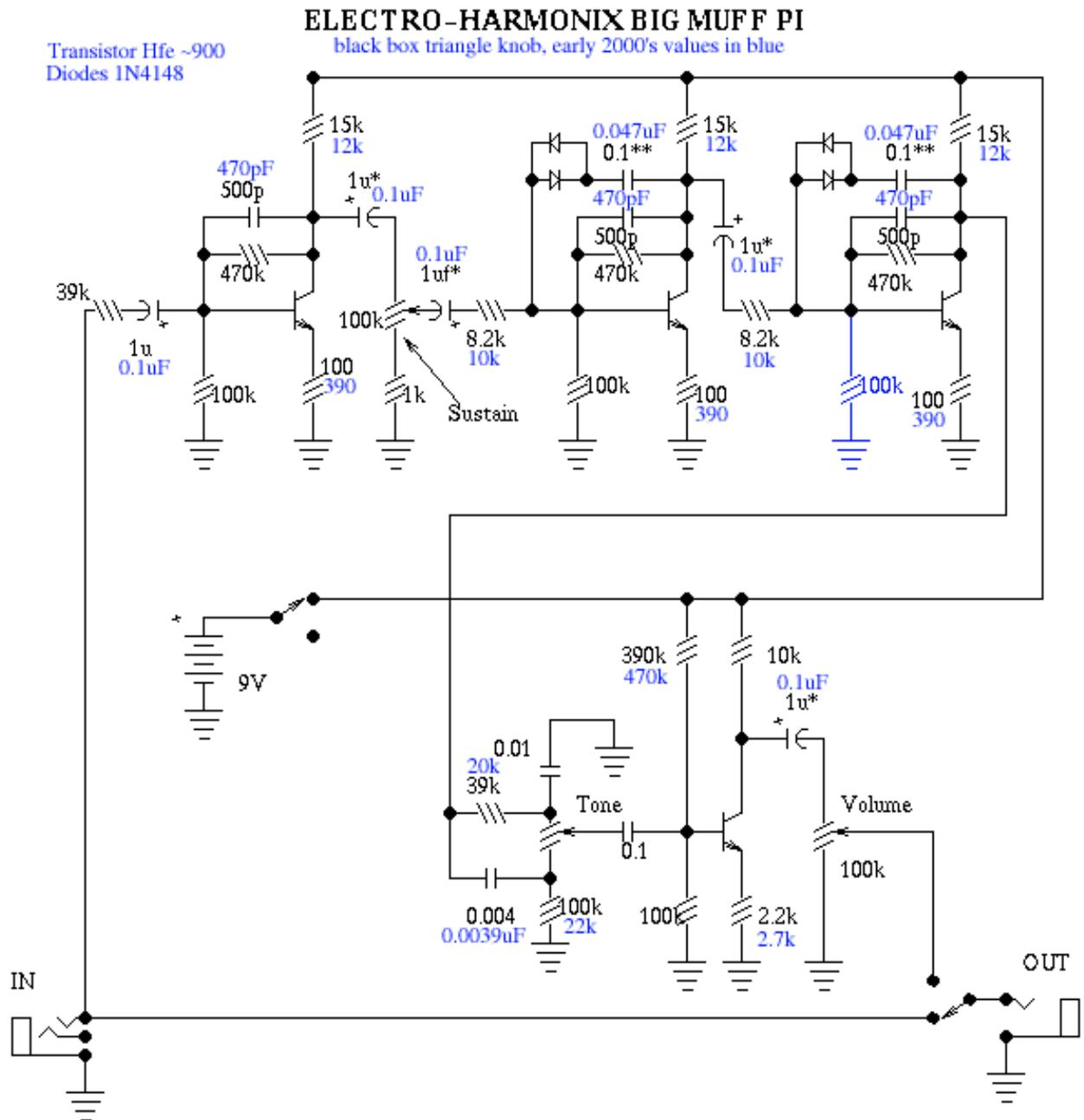
The EH Big Muff Pi would probably be improved by modern input-jack power switching and a DPDT bypass switch. This is the original schematic. The diode and transistor types are unknown. Probably any high gain NPN and 1N914s work. Coupling caps marked by a \* have been reported to sound better if changed to 0.1uf as have the \*\* marked ones if changed to 1.0uf. Has 22uF power supply bypass cap also.
