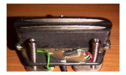
Now the pickup is ready to be installed on the bridge of your Telecaster without any wood-work on your guitar-body...
