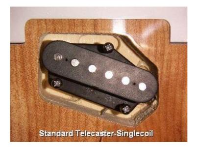
As you can see on this picture the new humbucker doesn't fit in this Telecaster because of its usual "mounting-ears" left and right of the pickup - just too big for this shape...
