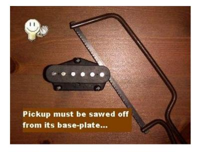
The first step is to remove the old pickup completely from its mounting-plate
